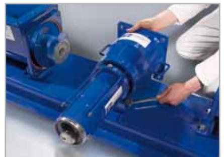
**6. Unscrew the rotor from the stator**
