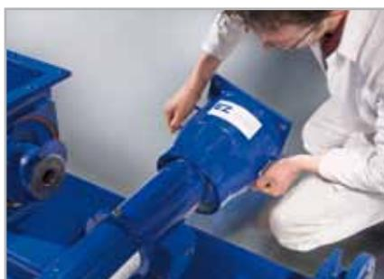
**8. Remove the stator**
