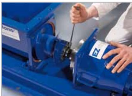
**4. Unscrew the tie bars and pull the tie bar assembly away from the discharge flange**
